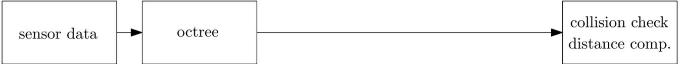
(b) By supporting the collision or distance query directly with the sensor data represented as octree, we no longer need the long conversion pipeline from octree to broad phase structures and thus can completely avoid the main overhead when preparing the sensor data for actual queries.
