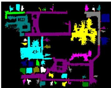
Figure 2: Regions in the topological map. Doorways are special regions, indicated in red. The map is derived from a metric map constructed from laser data.
