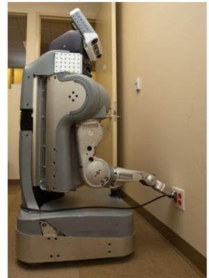
Figure 1: PR2 plugging in to a standard outlet.
