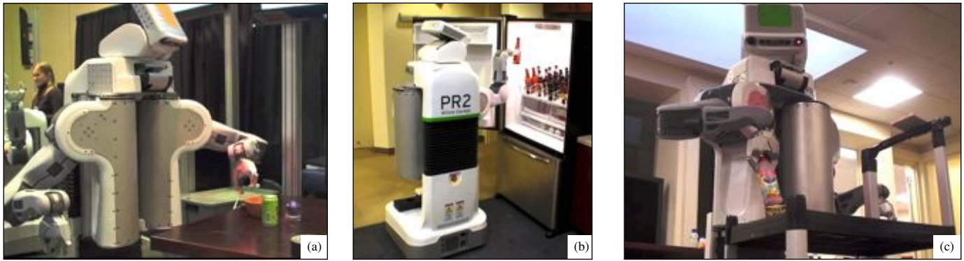
Fig. 13. Applications of our system (from left to right): (a) A pick and place application for moving objects. (b) A beverage retrieval application. (c) The PR2 using a cart to carry objects in a cluttered office environment.
