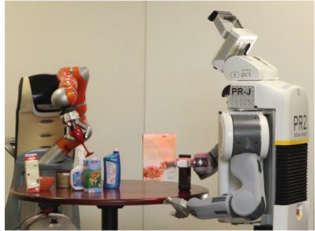
Fig. 1. The PR2 (right) and the Care-O-Bot (left). Both robots are executing a tabletop pick and place task using the approach described in this paper.
